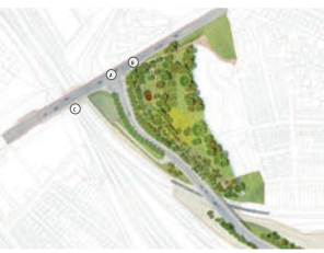
A. A new junction at Water End. B. New pedestrian and cycle crossing facilities and existing segregated cycle provision. C. New pedestrian and cycle bridge to the east of the Water End Road Bridge.
