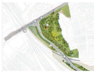
A. A new junction at Water End. B. New pedestrian and cycle crossing facilities and existing segregated cycle provision. C. New pedestrian and cycle bridge to the east of the Water End Road Bridge. D. Creation of a new bridge over the East Coast Main Line. E. New layout of accessible paths linking adjoining areas through the Millennium Green.
