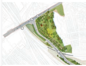
A. A new junction at Water End. B. New pedestrian and cycle crossing facilities and existing segregated cycle provision. C. New pedestrian and cycle bridge to the east of the Water End Road Bridge. D. Creation of a new bridge over the East Coast Main Line.
